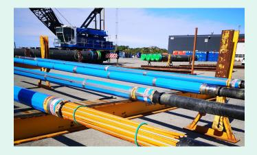
FlowTrace (patented) estimates zonal contribution per producing zone as fractions of the total well production. By deploying tracer rods in custom made tracer carriers as part of the completion string, the benefits of FlowTrace are:
